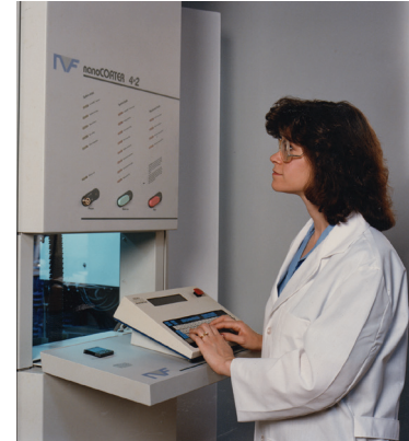
Nanocoater 4.2 - Designed, built and tested this lens coating machine for LensCrafters in 1985. The machine coats eyeglasses to protect them from smudges and damage.
